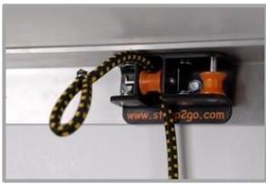
**STEP 3:** Mount the elastic rope to the wheel in the middle of the aluminium piece by pushing the loop of the elastic through the bottom side of the hole.
