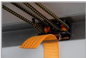
**STEP 6:** Mount the strap alongside the back of the hook. Ensure that the hook is in properly positioned so that the strap is positioned as close to the side as is possible.
