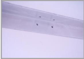
**STEP 1:** Drill 2 holes of 6.2 mm at the place where you want to attach the aluminium piece. This can be done **at the side** as well as **on top** of the profile. In case M6 bolts are to be screwed into the aluminium, then drill 2 holes of 5 mm and use a M6 tap for cutting a thread into the profile
