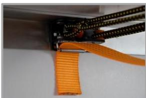
**STEP 7:** Pull the strap to aluminium piece 2 and push it trough the hook via the upper side.
